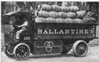
The truck above—a five-ton Atlantic—is a good example of the heavy duty electric vehicle. Trucks of this type are capable of traveling fifty to sixty miles on one battery charge. Below is the chassis of a one-ton truck of the same make
